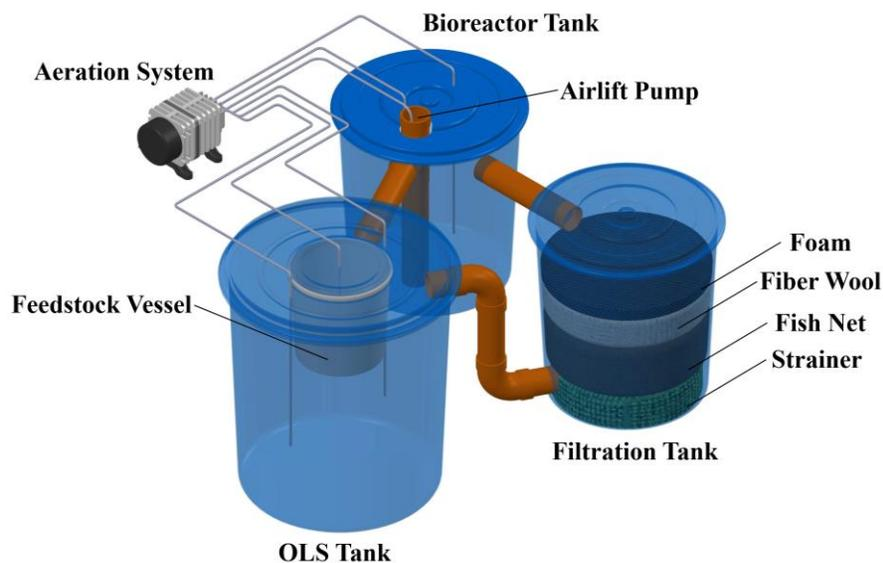
**Figure 3.** Design of organic fertilizer bioreactor for production of organic liquid solution
