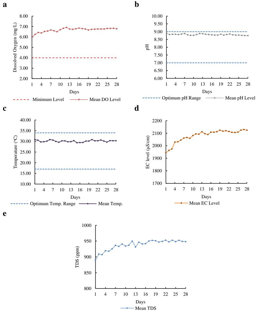
**Figure 4.** Trend of daily mean values of dissolved oxygen level (a), pH level (b), temperature (c), total dissolved solids (d), and electrical conductivity (e) of organic liquid solution using organic fertilizer bioreactor
