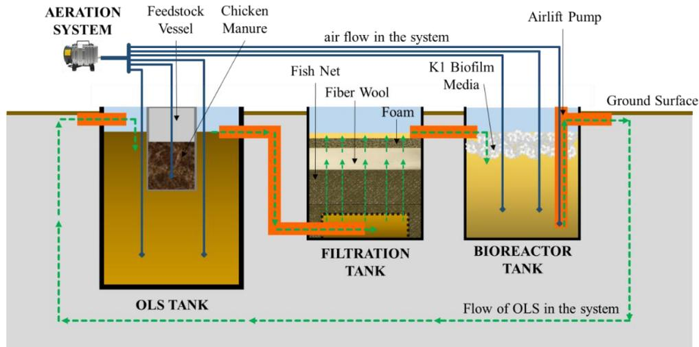
**Figure 1.** Schematic layout of the developed organic fertilizer bioreactor
