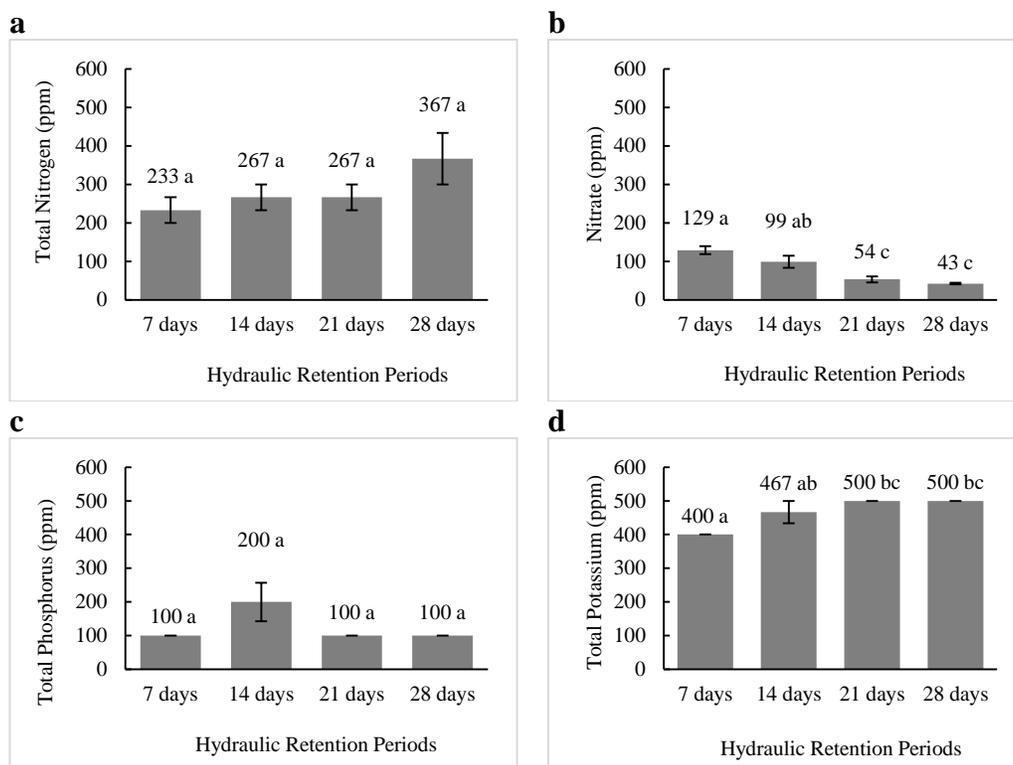
**Figure 5.** Quality of organic nutrient solution produced at different hydraulic retention periods using organic fertilizer bioreactor. Total Kjeldahl Nitrogen (a), Nitrate (b), Total Phosphorus (c), and Total Potassium (d). Different letters indicate statistically significant differences ( $p < 0.05$ ). The error bar represents the standard error of the mean
